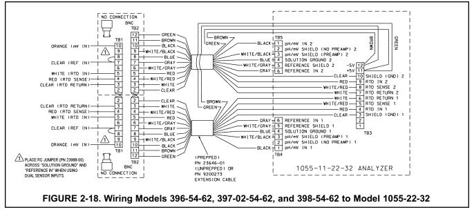
See below for wire functions for Models 396VP and 398VP. The Variopol connector cable part numbers are PN 23645-06 (with BNC) and PN 23645-07.
